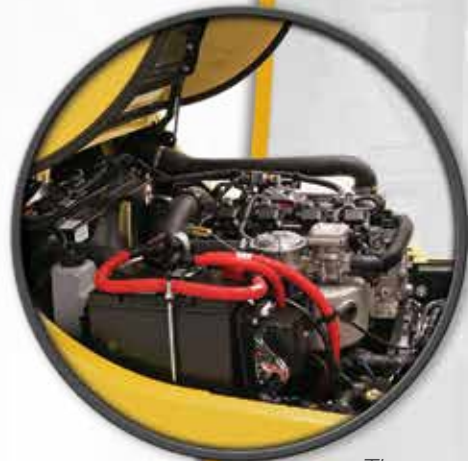
Three engine and two transmission selections available (PSI 2.4L LPG shown)
