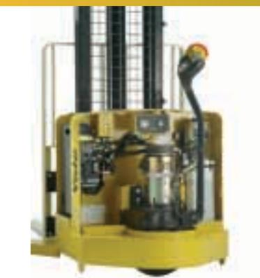
The MSW-E is designed for easy service access and maintenance. One power contactor reduces maintenance. The drive unit combines an integrated steer bearing and string guard to provide low maintenance and high up-time. The MSW-E comes standard with a low battery lift interrupt.
